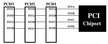
Figure 3-7 The Combination of PCI INT#lines
