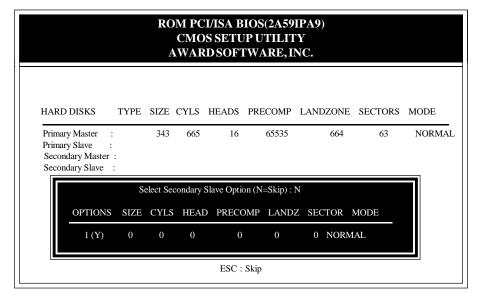
**Figure 3-9 IDE HDD AUTO DETECTION**
