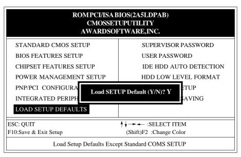
Figure 3-8LOAD SETUP DEFAULT
