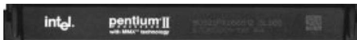
Intel Pentium II Processor in an SEC Cartridge (233-400MHz 256/512KB L2 Cache)
