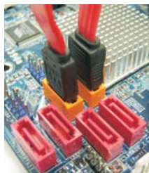
Connect the SATA data cables to both orange SATAII connectors (SATAII_6 (Port5) and SATAII_5 (Port4))
