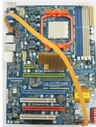
Connect the SATA data cable to the eSATAII connector (eSATAII_TOP)
