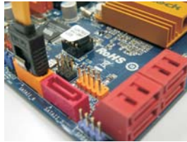
Connect the SATA data Cable to the orange SATAII connector (SATAII_6)
