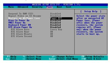
Suspend to RAM (S3): This field allows you to select whether to auto-detect or disable the ACPI Suspend-to-RAM feature. Select [Auto] will enable this feature if the system supports it.
