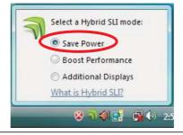
Step 8. Click the desktop. Then your system is switched to HybridPower™ mode (Save Power). \_\_\_\_\_
