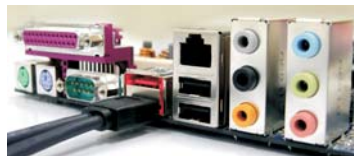
Connect the other end of the eSATAII device cable to eSATAII port of the I/O shield
