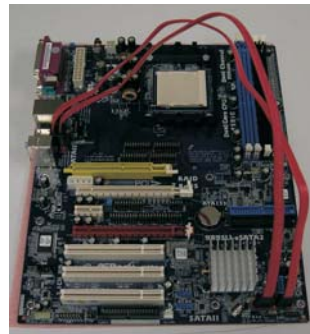
Connect the SATA data cables to both red eSATAII connector (eSATAII_BOTTOM) and orange eSATAII connector (eSATAII_TOP)
