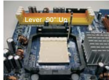
STEP 1: Lift Up The Socket Lever
