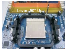
STEP 1: Lift Up The Socket Lever
