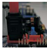
Connect the SATA data cable to the red SATAII connector (SATAII_RED)
