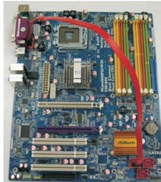
Connect the SATA data cable to the eSATAII connector (eSATAII)
