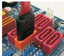
Connect the SATA data cable to the orange SATAII connector (SATAII_6 (Port5))
