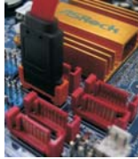
Connect the SATA data cable to the orange SATAII connector (SATAII_6 (Port5))
