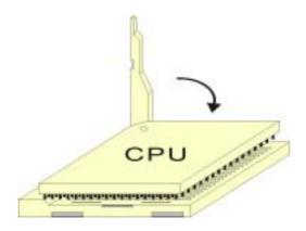
Press the lever down. Then Put the CPU fan on the CPU socket and clasp it with the socket. When the CPU fan is fixed to the CPU socket, put the fan's power port into the CPUFAN. After finishing all these steps, the CPU is ready for use.
