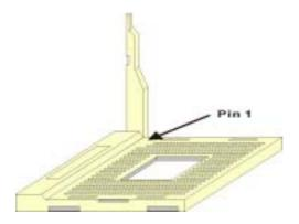
2. Find Pin-1 in the socket and look for the white dot or cut edge in the CPU. Match Pin-1 with the white dot/cut edge then insert the CPU.
