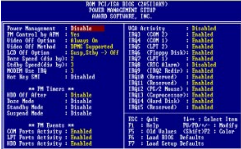
Power management setup
